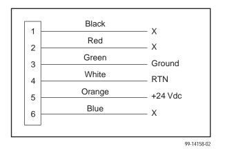
+24 Vdc Power Supply Pinouts
